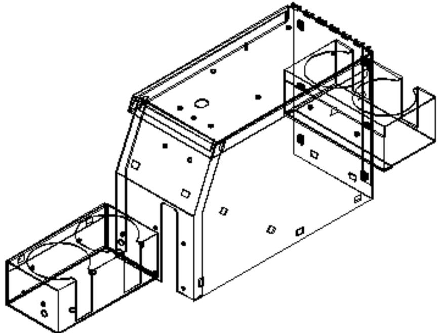
2. Pull the emergency brake all the way up and place the console between the seats in the final mounting position desired. **NOTE:** If the emergency brake pulls up more than about 45 degrees it should be adjusted by a qualified professional prior to installation of your Tuffy console.
