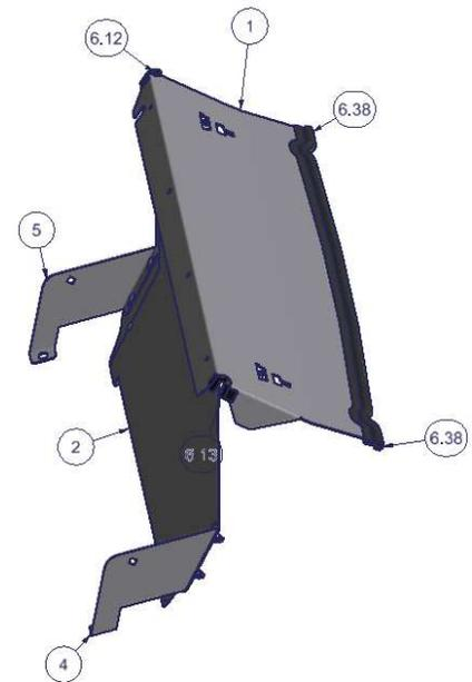
29. Be sure the #2 Front Panel is aligned, centered, and positioned in the vehicle as desired. Verify the #9 OEM Rear Storage Cover (or #143 Tuffy Cubby Cover, if installed) has adequate clearance for operation. Be sure the #2 Front Panel is pushed as far downward as possible for a tight fit to the cargo floor. (Figure 4)
