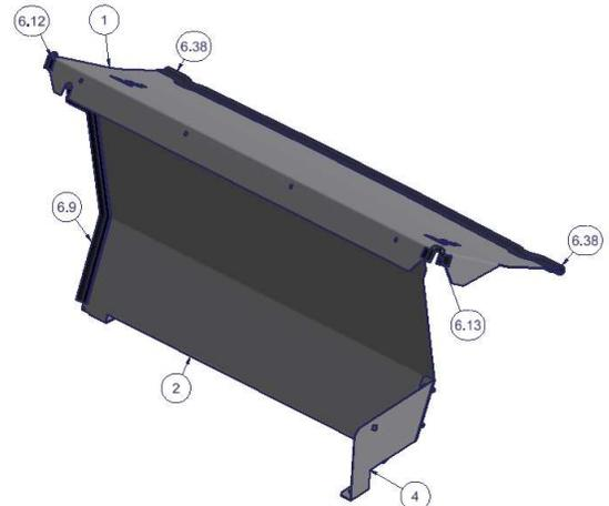
22. Be sure the #2 Front Panel is aligned, centered, and positioned in the vehicle as desired. Verify the #9 OEM Rear Storage Cover (or #143 Tuffy Cubby Cover, if installed) has adequate clearance for operation. Be sure the #2 Front Panel is pushed as far downward as possible for a tight fit to the cargo floor. (Figure 4)
