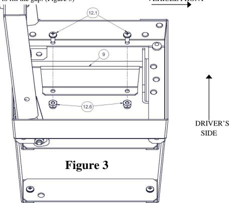
8. Push the Insert as far to the driver's side of the vehicle as possible, and install the #8 Right Plate using (2) #12.1 Machine Screws and #12.6 Nylock Nuts. The upper flange will slip between the upper collar of the Insert and the console interior, in order to fill the remaining gap. (Figure 4)
