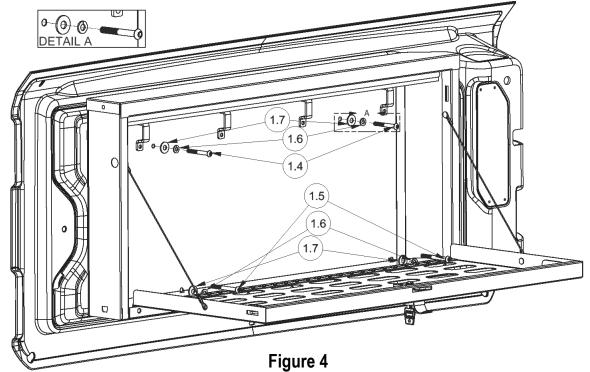
7. Tighten mounting hardware to 8 ft-lbs(10 N-m).
