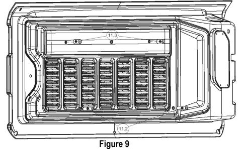
13. While holding the #365 Storage Box in place, insert the mounting hardware through the mounting holes of the #365 Storage Box in the sequence shown in Figure 10. #1.3 Screws (2") are used in the upper mounting holes, and #1.5 Screws (2 3/8") in the lower holes. *NOTE: This step is most easily accomplished with help, or another means of supporting the lockbox at the correct elevation.*
